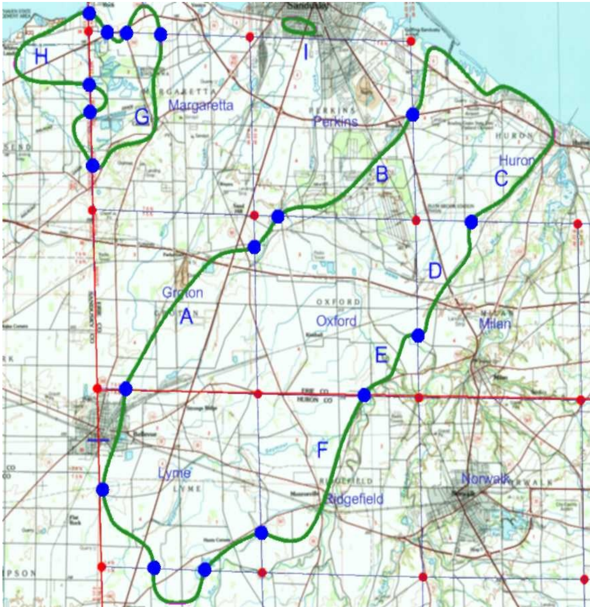
Fig. 4. Prairie borders determined from surveyors' field notes. Blue dots are recorded prairie edges along township borders. Red dots are township corners.
